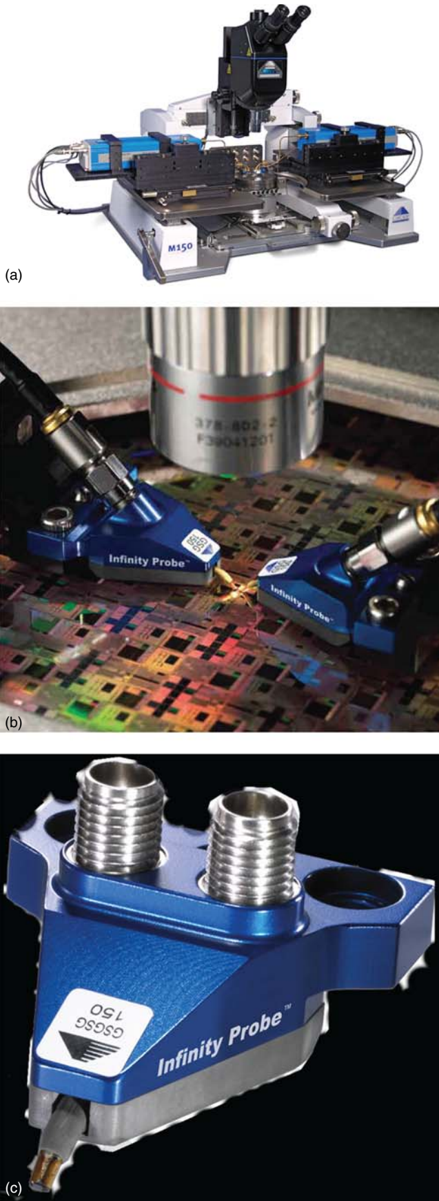
Figure 15.9. Probe station (a), on-wafer probe setup with single-ended probes (b), and a differential probe (c). (Courtesy of Cascade Microtech, Inc.)
